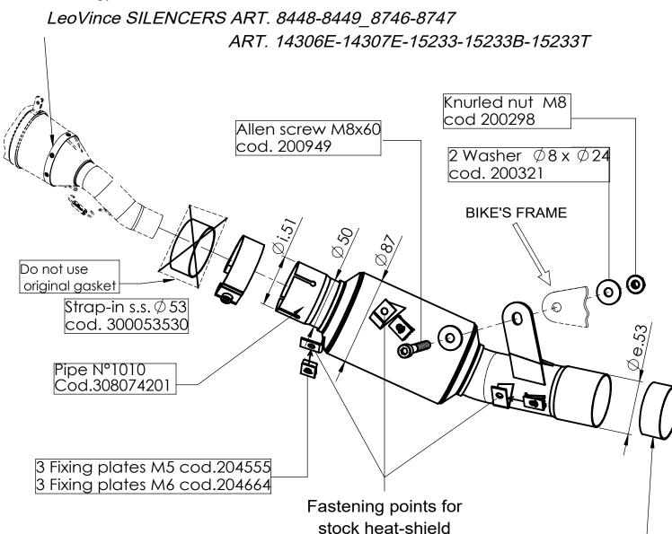
Disconnect the control cables from the exhaust valve on the actuator side; by removing the original link pipe with the catalytic converter, also the valve connected to the link pipe and the cables are removed.
